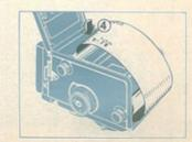
Inserting the film: Pull out the film knob (1) at the lower spool chamber and insert the roll of film. Insert the right-hand end first. Let the film knob spring back fully.
